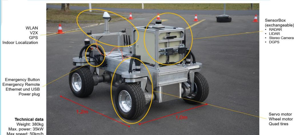
Fig. 1. Smart Physical Demonstration and Evaluation Robot (SPIDER)
