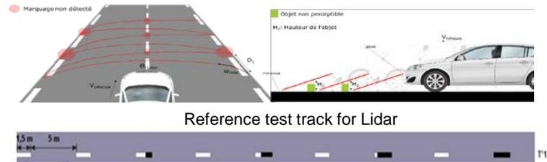
Reference test track for Lidar
